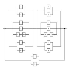
Figure 5. Reliability network for a fire detection and alarm system.
