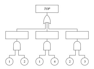
Figure 2. Equivalent fault tree created based on minimal cut sets [3].
