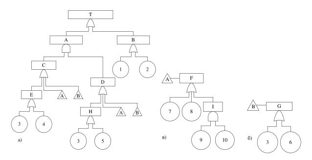
Figure 3. Fault tree of a fire detection and alarm system for qualitative analysis.
