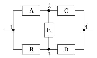
Figure 1. Bridge structure reliability network.
